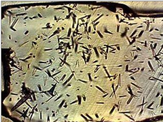
Etched fission tracks from 238 uranium in apatite. track lengths are approximately 17 microns.
